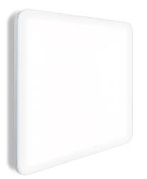
Size 430 mm Fitting LED 18 W Performance level 2100 lm Colour temperatures 3000 K, 4000 K Light distribution Lambertian Lighting control Switchable, DALI Installation options Wall, ceiling or pendant installation
