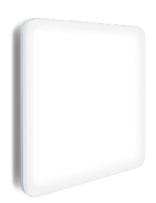
Size 330 mm Fitting LED 13 W Performance level 1200 lm Colour temperatures 3000 K, 4000 K Light distribution Lambertian Lighting control Switchable, DALI Installation options Wall, ceiling or pendant installation
