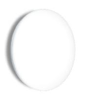
Size Ø 330 mm Fitting LED 17 W Performance level 1100 lm Colour temperatures 3000 K, 4000 K Light distribution Lambertian Lighting control Switchable, DALI Installation options Wall, ceiling or pendant installation
