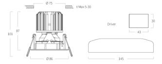
A small recessed downlight with two light distributions and one colour temperature, with an IP44 rating. Provides an elegant general lighting solution for corridors or communal areas.
